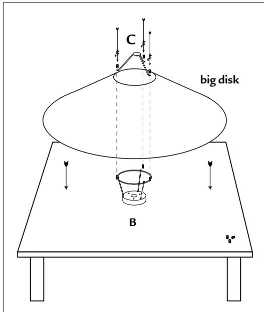
5. Insert element **C** and tighten the three screws on element **B**.
