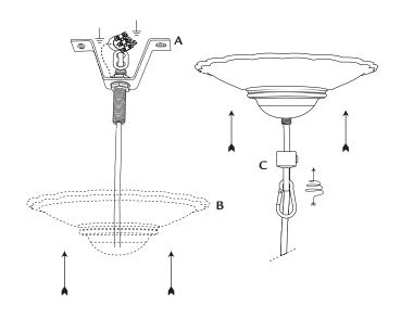
5. Screw the hook  ${\bf C}$  onto the nipple and tighten securely.
