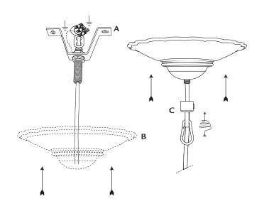
5. Screw the hook  ${\bf C}$  onto the nipple and tighten securely.
